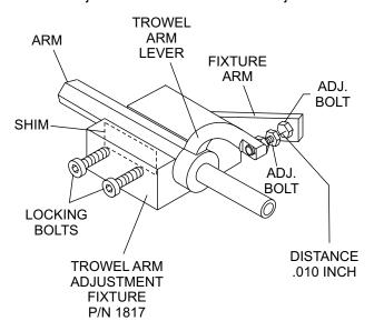
Figure 44. Trowel Arm Adjustment Fixture Components
